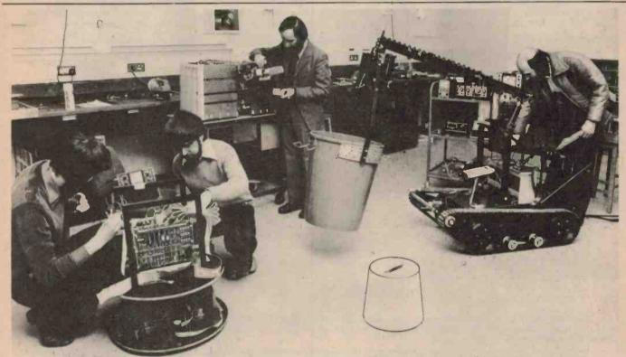
Fig. 1. Projects of the Warwick University Robot Laboratory. Project on the left uses an inboard microprocessor. At the rear is a hand-like short arm manipulator. The tracked vehicle is originally sold as the army bomb-disposal unit — it acts as a ready made vehicle to conduct research on. (Keystone Press Agency).
