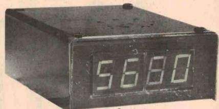
The usual solution is to use a 100 rev resolution and a sample time of 0.3 seconds (on 4 cylinders). We considered this inadequate which is why we have not published a design until now.
